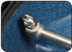
Welded jet housings.
