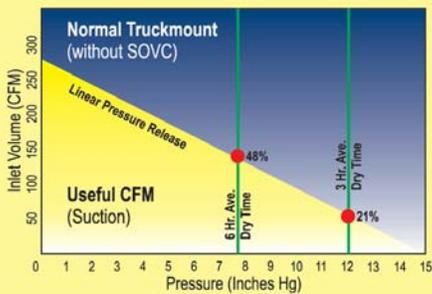
As the chart to the left illustrates, the spring and disc pressure relief valve used on most truck mounts begins to open the moment the truck mount is started. The result is an immediate loss of CFMs. As the pressure is increased, CFMs continue to decrease cutting suction by 80% at 12" Hg.
