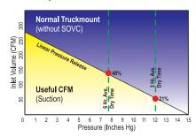
The SOVC kit replaces the manual relief valve with an electronically-controlled valve system that safely maximizes the suction power of your truck mount. As the chart below shows, SOVC delivers a massive power boost and cuts dry times dramatically.
