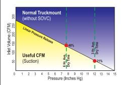
As the chart to the left illustrates, the spring and disc pressure relief valve used on most truck mounts begins to open the moment the truck mount is started. The result is an immediate loss of CFMs. As the pressure is increased, CFMs continue to decrease cutting suction by 80% at 12" Hg.
