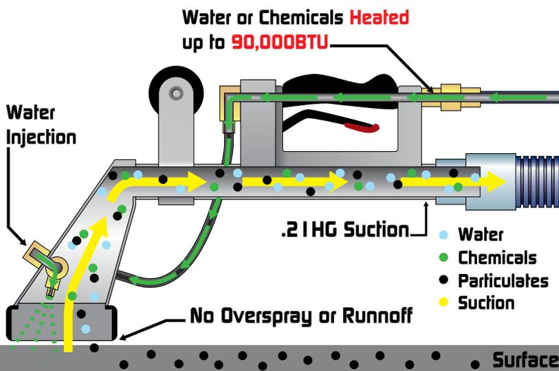
**WHAT IS CLEAN AND CAPTURE?** Clean and Capture is a proprietary technology of PowerPlus Professional Cleaning Solutions that utilizes heat, suction, pressure, and chemical properties to achieve a decontamination solution second to none. The PRODIGY BIO is completely integrated with this system that can provide a safe, inexpensive, way to reclaim contaminated areas.
