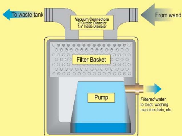
**Explanation:** The Auto Pump-Out connects inline with your vacuum hose. The 1,500 gallon per hour pump pulls waste water through the stainless steel filter and pushes it out the filtered water output valve. The Auto-Pump disposes almost all of the waste water before it enters the waste tank enabling you to work all day without stopping to drain your tank.
